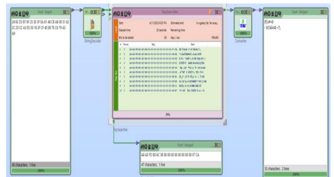
Fig.3. The developed scheme of the attack on the AES cryptosystem
