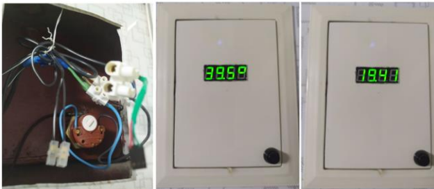
Fig. 2. Connecting the sensor to the container and controlling the temperature via buttons on the container itself.
