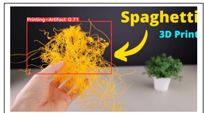
Fig.8. YOLOv8-based valid detection of defects at the test image.
