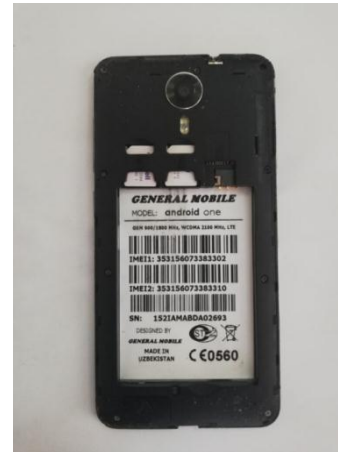
Fig.2. Definitions of the International Mobile Equipment Identifier code on the case of a mobile device
