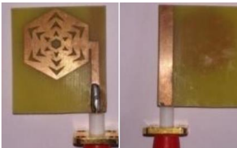
Fig. 2. The prototype of a hexagonal fractal antenna [11]
