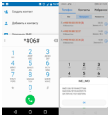
Fig.1. Determination of the International Mobile Equipment Identifier code of a mobile device by the number combination * # 06 #
