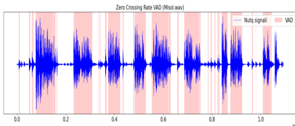
Fig. 5. Time series and VAD results based on Zero crossing rate and energy
