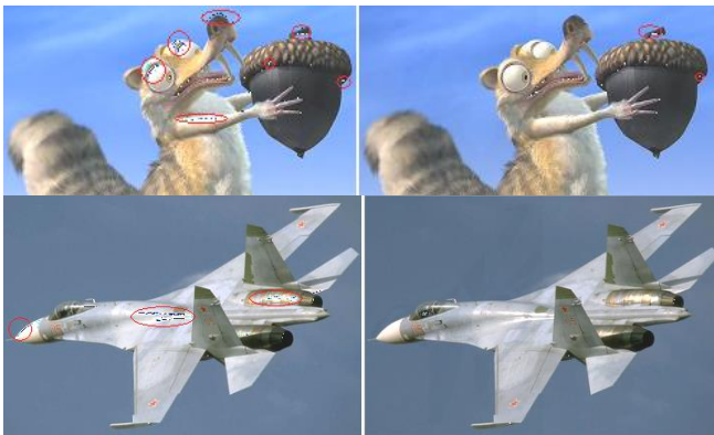
Fig.9. Areas of color distortions, introduced by the LeGall (5.3) and Deslauriers-Debuc (13.7) filters in the images.
