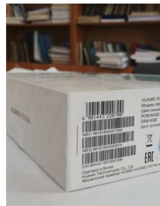
Fig.3. Determining the IMEI code by packaging 4) Definition of the IMEI code in the phone settings (Fig.4).
